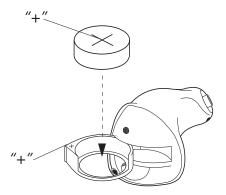
The batteries for the hearing instrument are quite small, and it may cause difficulty seeing the battery and battery door markings. A magnifying glass and good lighting may be helpful. When the battery voltage/power decreases to a certain level, the instrument will stop amplifying and emit a soft beeping signal. This signal will continue for about one minute and then the instrument will be automatically switched off. Therefore, it is recommended that you keep a spare battery on hand.
