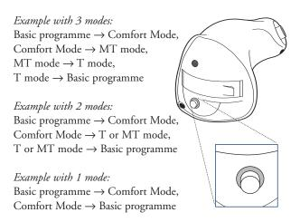
You can always return to the basic programme by turning your instrument off and then on again (see "On/Off Function") or by placing it in stand-by mode and then returning to its normal function mode (see "Stand-by Function" on the next page).
